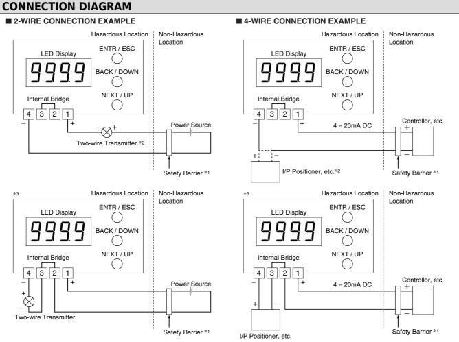
\*1. A safety barrier must be installed for the intrinsic safety.
