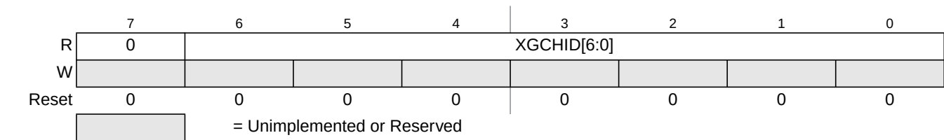
Figure 6-4. XGATE Channel ID Register (XGCHID)
