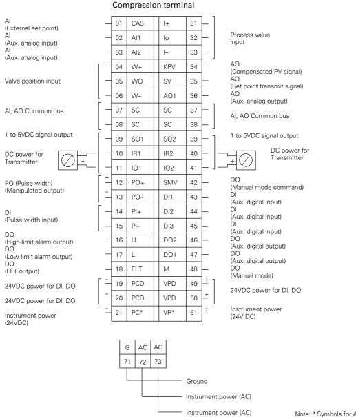
Note: \* Symbols for AC instrument power are VPO, PCO. Output: approx. 24V DC (0.1A, max.)
