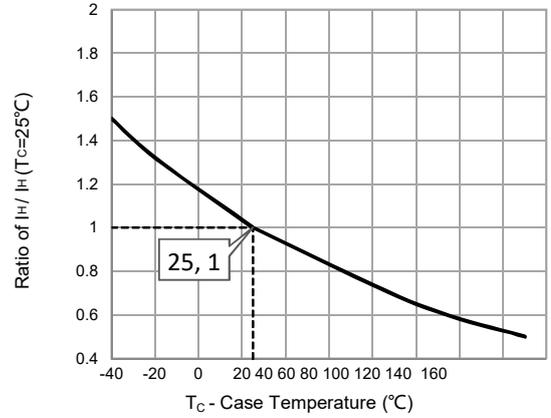
Fig. 2 - Normalized DC Holding Current vs. Case Temperature
