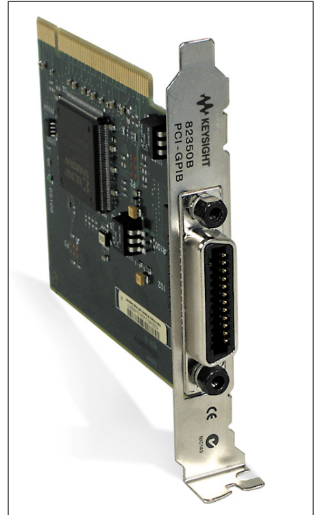
82350B PCI high-performance GPIB interface card
