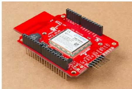
Shield with stackable headers installed.
