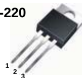
1.Gate 2. Drain 3. Source
