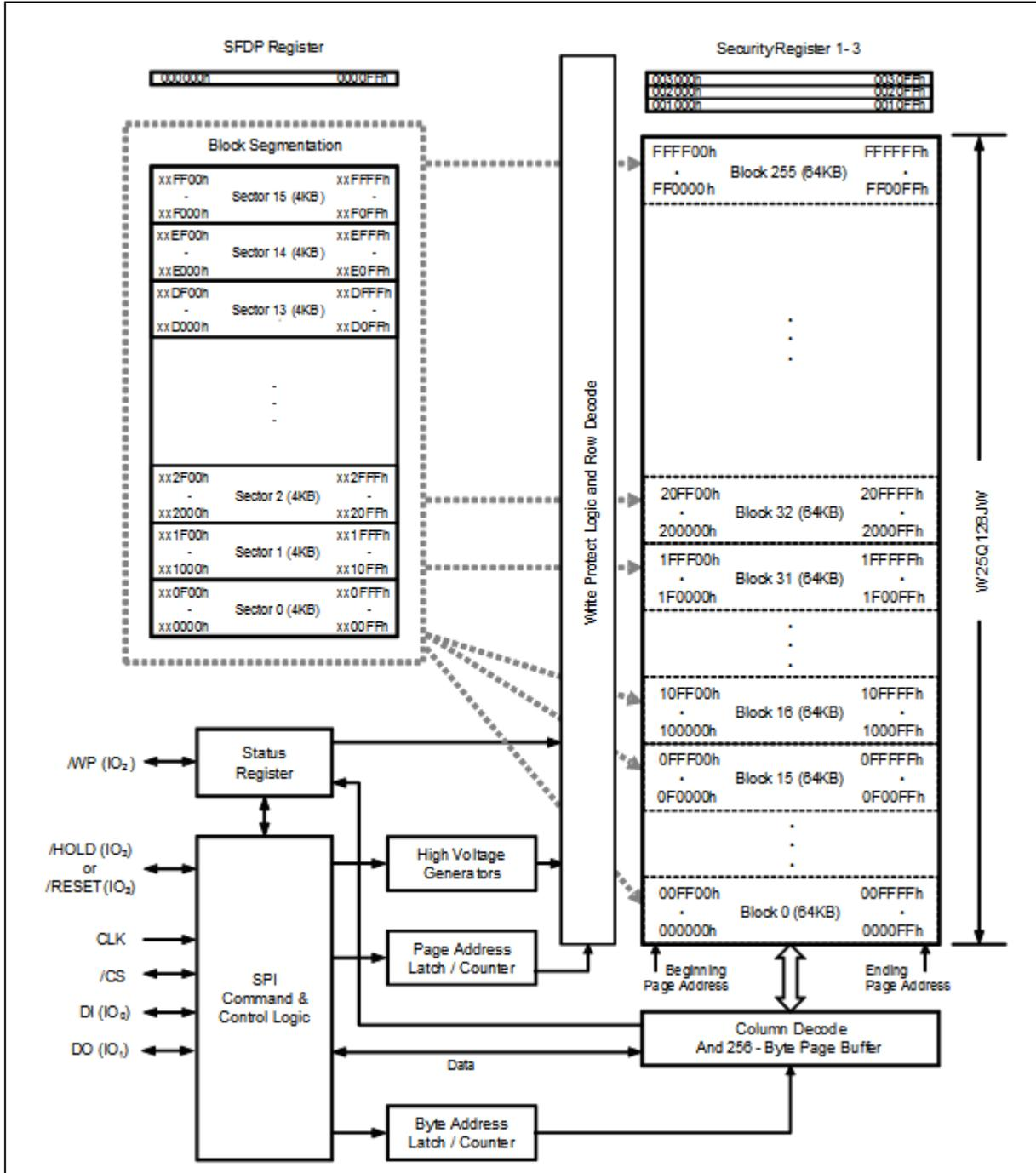
Figure 2. W25Q128JW Serial Flash Memory Block Diagram
