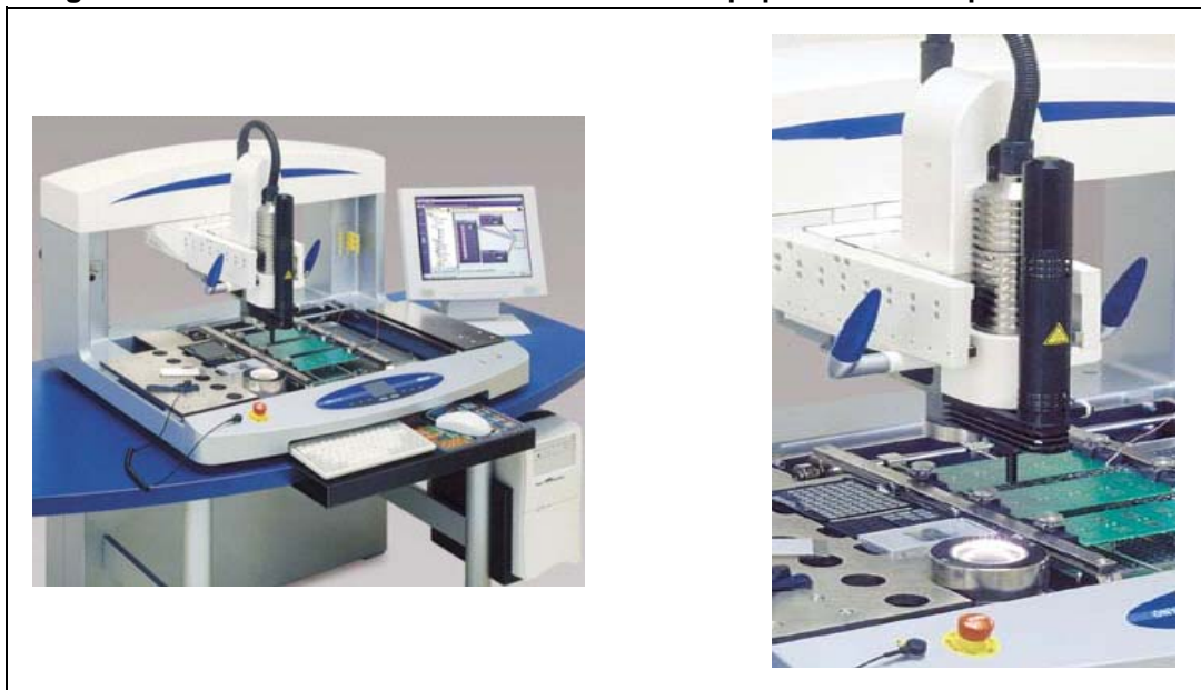
Figure 11. Comintec ONYX32 - Semi-automatic equipment for component rework
