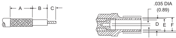
50 Ohm Contact (RG-196U) (assembly steps 1, 2, 3, 4, 5 & 8)
