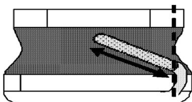
5 Exectrde appearance criterion for exposed wire
