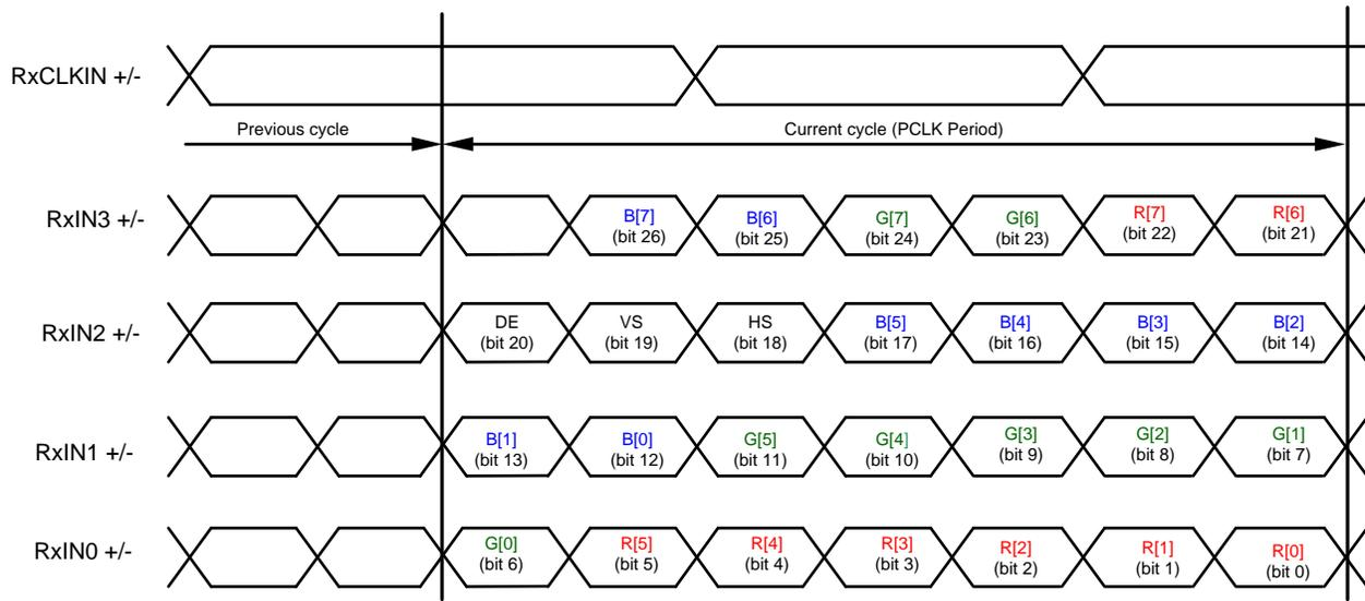
Figure 20. FPD-Link Mapping: MSBs on RxIN3 (MAPSEL=H)
