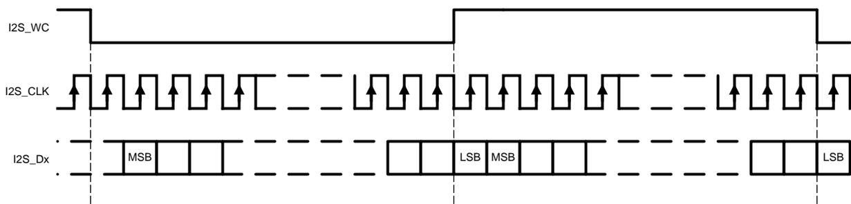
**Figure 18. I<sup>2</sup>S Frame Timing Diagram**
