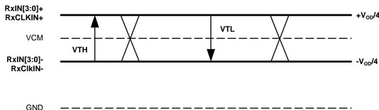
Figure 1. FPD-Link DC V<sub>TH</sub>/V<sub>TL</sub> Definition
