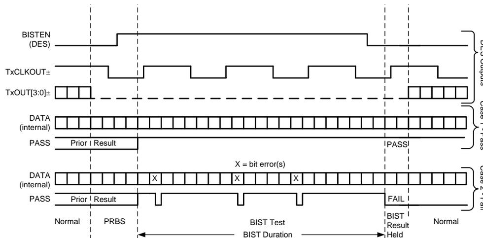
**Figure 15. BIST Waveforms**
