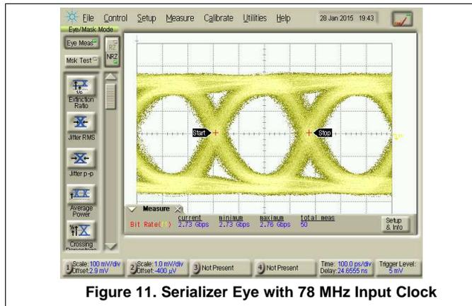
Figure 11. Serializer Eye with 78 MHz Input Clock
