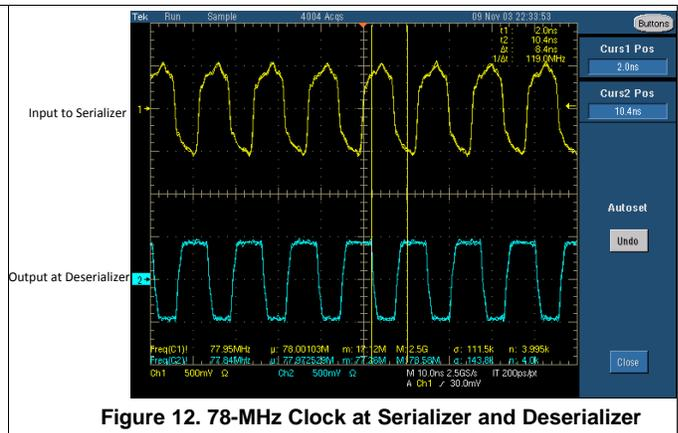
Figure 12. 78-MHz Clock at Serializer and Deserializer
