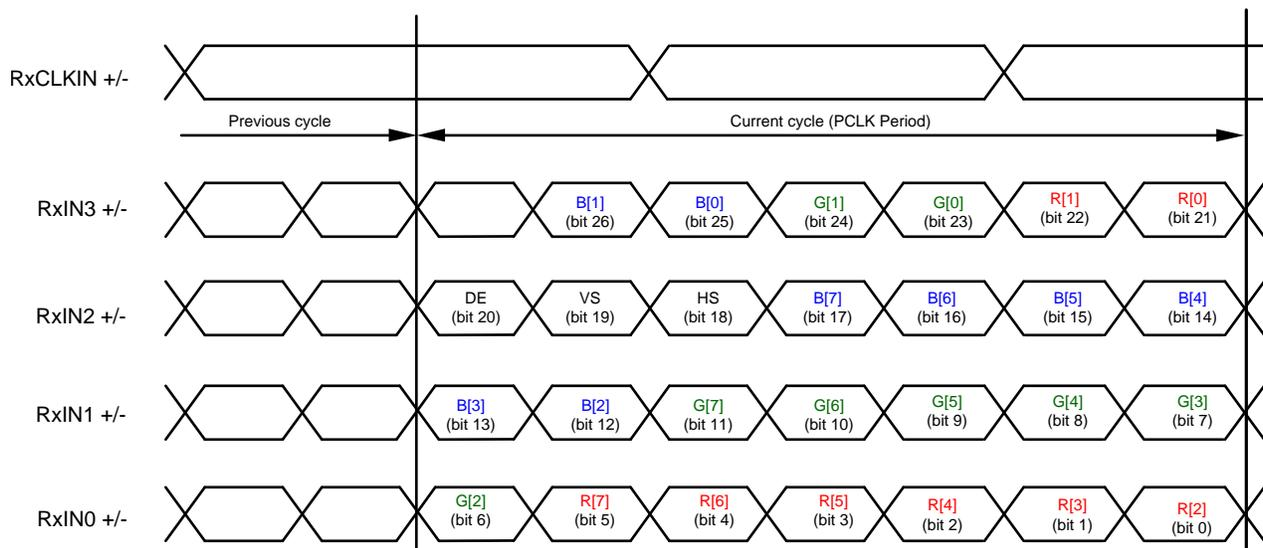
Figure 19. FPD-Link Mapping: LSBs on RxIN3 (MAPSEL=L)
