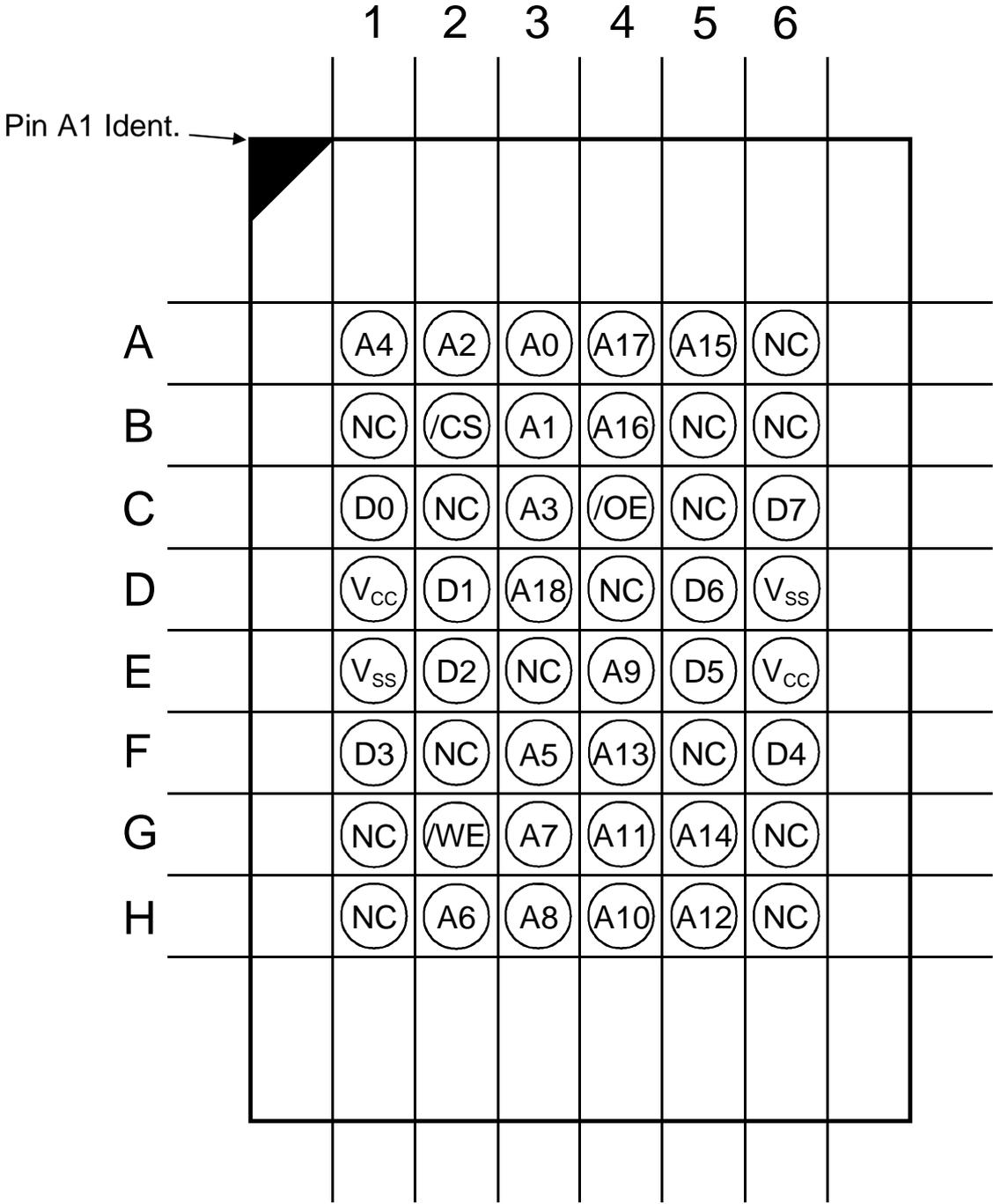
Note : Pinout shows top view,
