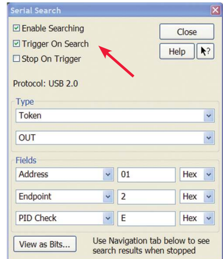
USB Trigger Setup Choose triggers from a broad range of USB protocol, including token, data, handshakes, special and error types.
