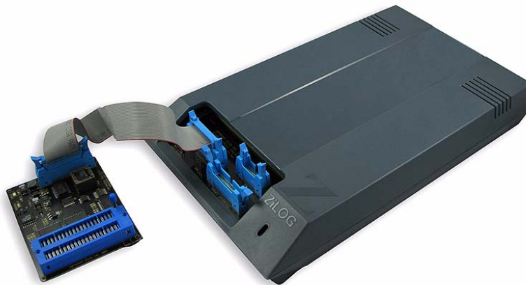
Figure 5. OTP Programming Adapter (Included with Crimson ICE)
