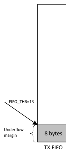
Figure 16 Example of TX FIFO at Threshold
