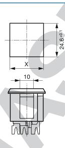
Panel thickness X 0.8 - 1.2 mm: 24.6 mm 1.3 - 1.6 mm: 24.8 mm
