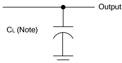
Note :  $C_L$  includes probe and jig capacitance.
