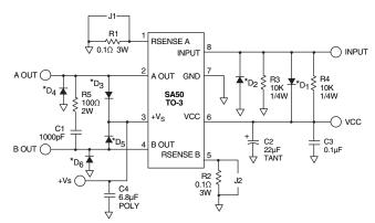
\* D<sub>1</sub> and D<sub>2</sub> – Input protection, high speed such as IN4148. D<sub>3</sub> through D<sub>6</sub> – Flyback protection, high speed (<200nS). Solder as close to SA50 as possible.
