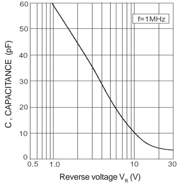
Fig.2 Capacitance Vs. Reverse voltage
