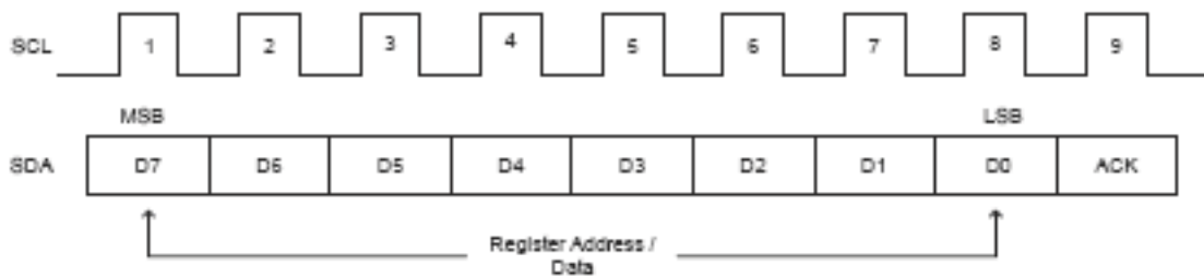
Figure 4: I 2 C Register Address and Data Bit Map;
