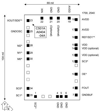
Note: ^: Internal pull-up resistor (120kΩ for SD0, 30 kΩ for SC0-SC2, SD1, M0-M2 and OE). The internal pull-up resistor results in a default high value when no pull-down resistor is connected to this pin.
