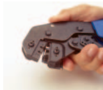
4. Partially (usually the first click) Cycle the hand tool assuring that the upward thrusting tails of the contact has started engaging with the top jaw of the tool. (There is a slight tendency for the contact to roll out of vertical alignment.)
