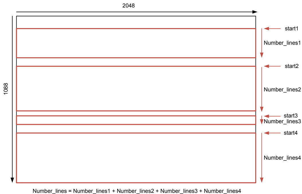
FIGURE 39: EXAMPLE OF 4 MULTIPLE FRAMES READ-OUT
