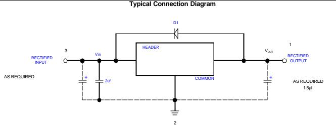
Note: D1 should be installed for input safety.
