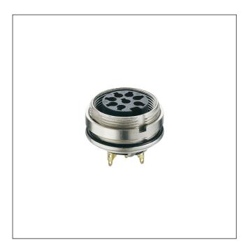
Chassis socket acc. to AISG specification and IEC 61076-2-106, IP 68, with threaded joint and solder terminals, for back side mounting
