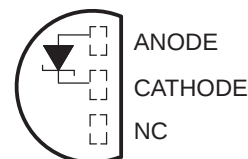
LP (TO-92/TO-226) PACKAGE (TOP VIEW)
