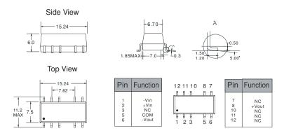
Note: All Pins on a 2.54mm pitch; all pin diameters are 0.50mm; all dimensions in mm.
