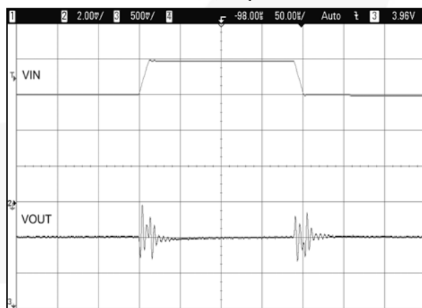
Figure 21. Line Transient V_{IN} = 3.7\text{ V} to 4.2\text{ V} , V_{OUT} = 2.5\text{ V} , 5\text{ }\Omega Load, 50\text{ }\mu\text{s/div} .
