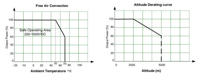
\*NOTE: Derating is indicated at natural convection. Sufficient air space around is needed.
