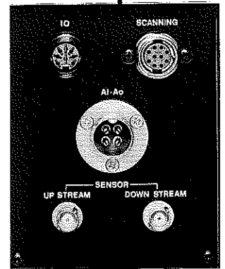
Connectors for sensor, analog input/output, personal computer interface, scanner
