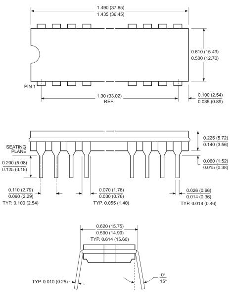
28-LEAD HERMETIC DUAL IN-LINE PACKAGE TYPE D
