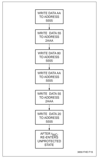
In the event the user wants to deactivate the software data protection feature for testing or reprogramming in an E<sup>2</sup>PROM programmer, the following six step algorithm will reset the internal protection circuit. After  $t_{WC}$ , the X28HC256 will be in standard operating mode.
