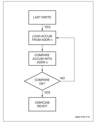
The Toggle Bit can eliminate the software housekeeping chore of saving and fetching the last address and data written to a device in order to implement DATA Polling. This can be especially helpful in an array comprised of multiple X28HC256 memories that is frequently updated. The timing diagram in Figure 4 illustrates the sequence of events on the bus. The software flow diagram in Figure 5 illustrates a method for polling the Toggle Bit.
