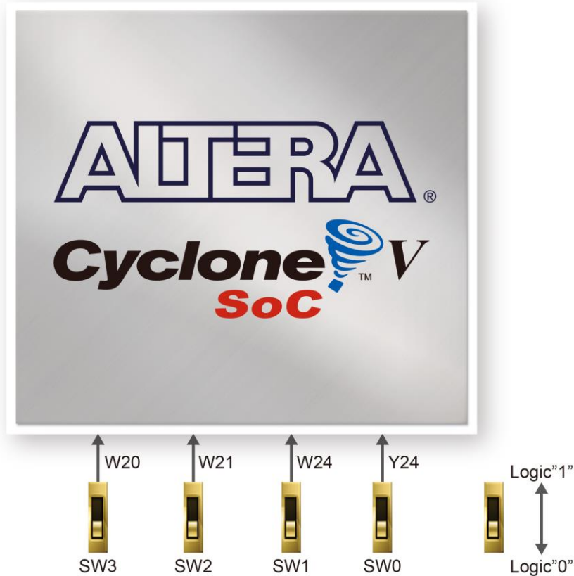
Figure 3-18 Connections between the slide switches and the Cyclone V SoC FPGA
