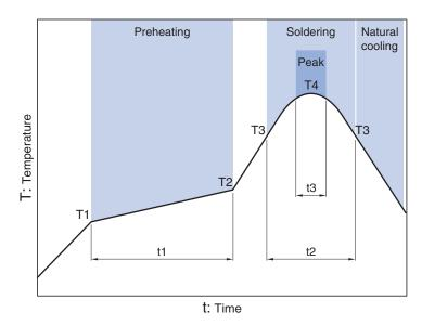
Preheating Soldering Peak Temp. Temp. Time Time Temp. Time T1 T2 T4 T3 150°C 180°C 60 to 120s 230°C 10 to 30s 245°C 5s max.
