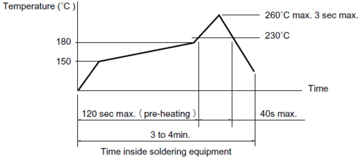
(1) The above temperature shall be measured of the top of switch. There are cases where PC board's temperature greatly differs from that of the switch, depending on the material, size, thickness of PC board's and others. Care, should be taken to prevent the switch's surface temperature from exceeding 260°C.
