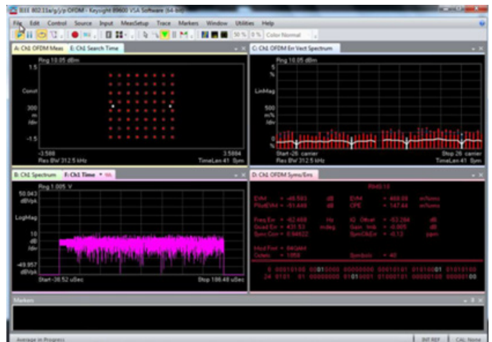
Using data acquired from S-Series, VSA shows an EVM for IEEE 802.11 QAM 64 of 0.47%.
