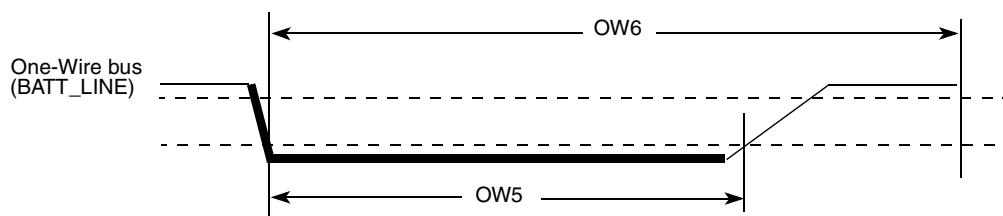
Figure 5. Write 0 Sequence Timing Diagram
