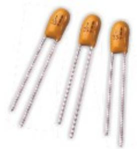
Small units with high stable performance, low current leakage and dissipation factor, stable frequency and temperature and long life, suitable for electronic communication, computer and military and so on. Operating temperature -55-125C, +85C With derating voltage. Capacitance range:0.047uF-680uF, DC Leakage Current(20C)  $I_o \leq 0.01C_R U_R$  or 0.5uA( Whichever is bigger), Life test: 1000hours
