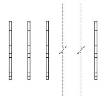
NOTE: CONTACTS ARE HELD IN A CARRIER FOR EASE OF ASSEMBLY
