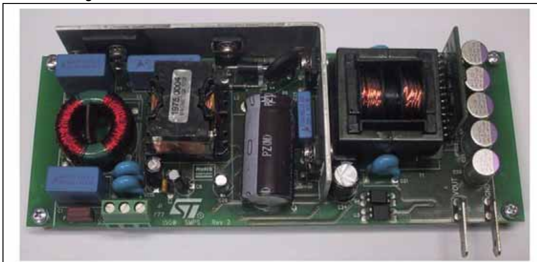
Figure 9. EVL6699-150W-SR 150 W SMPS demonstration board
