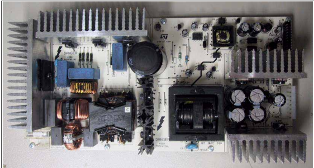
Figure 19. L6599 and L6563 400 W evaluation board (EVAL6599-400W-S)
