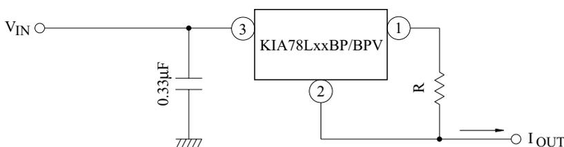
$$I_{OUT} = \frac{V_{OUT}}{R} + I_B$$
