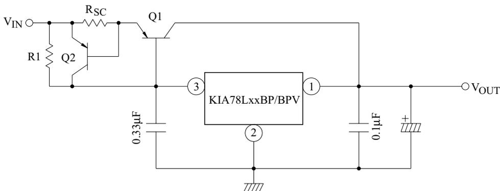
$$R_{SC} = \frac{V_{BE2}}{I_{SC}}$$
