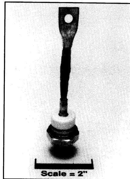
A180 (R) Silicon Rectifier 150 Amperes Average, 1600 Volts
