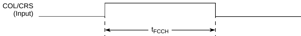
Figure 26. Ethernet Collision AC Timing Diagram (FCC)
