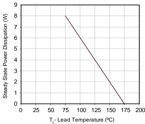
Figure 5 - Steady State Power Dissipation Derating Curve
