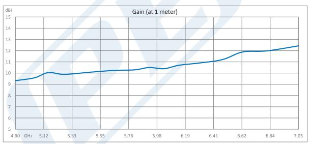
Click the following link (or enter part number in "SEARCH" on website) to obtain additional part information including price, inventory and certifications: WR-159 Waveguide Standard Gain Horn Antenna Operating From 4.9 GHz to 7.05 GHz With a Nominal 10 dBi Gain With CMR-159 Flange PE9860-10
