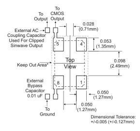
\* Do not route any traces in the keep out area. It is recommended the next layer under the keep out area is to be ground plane.
