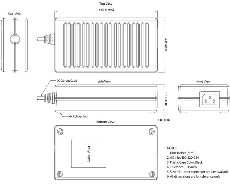
Standard output cable: AWM 2464 #16 AWG / 3C + SHIELDING, UL 80°C 300V VW-1, 1050mm
