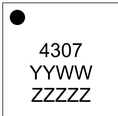
Figure 21. Top Marking Specifications
