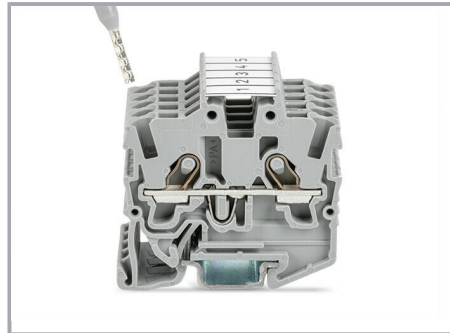
Insert ferruled conductors via push-in termination.
