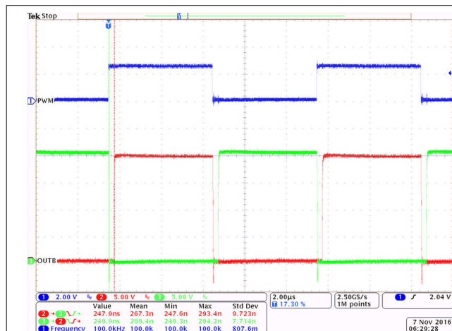
图 9-5. Bench Test Waveform for PWM and OUTA/B
